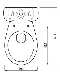
All dimensions are in milimetres unless otherwise stated. The information contained on this page was correct at date of issue. Fitting dimensions are provided as a guide only. Some variation may occur due to manufacturing tolerances. We pursue a policy of continuing improvement in design and performance of our products and so reserve the right to change specifications without prior notice.
